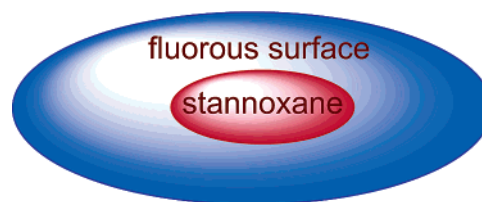
FIGURE 1. Double-layered structure of fluorous distannoxane.
